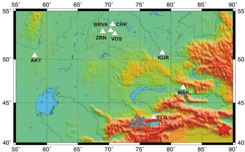
Location map of explosion epicenters and seismic stations from which records were used for processing. White triangles are the stations of the IGR NNC RK (KZNET), and grey triangles are KNET network stations. Red stars are the places of nuclear tests conducted at the LNTS.
