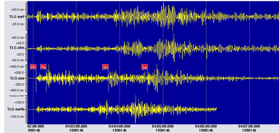
Comparison of station TLG vertical component seismograms. From top to bottom: surface explosion of 28 December 1966; atmospheric nuclear explosion of 17 June 1973,  $m_b=4.8$ ; underground nuclear explosion of 26 May 1990,  $m_b=5.5$ ; tectonic earthquake of 9 March 1975,  $m_b=4.6$ .
