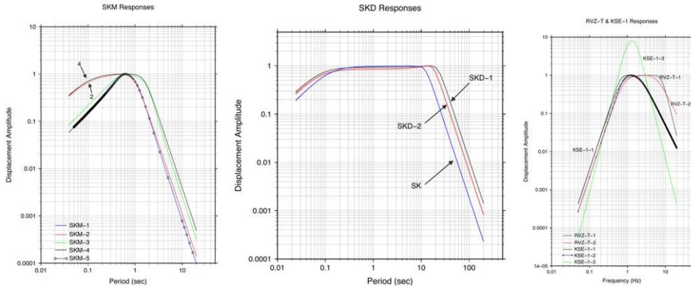
Typical responses of analog seismic stations in Central Asia
