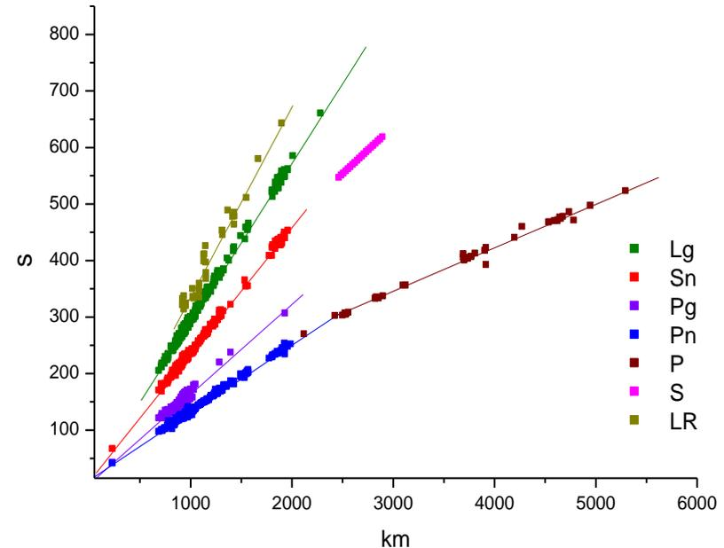
**Composite travel time curve for Lop Nor explosions analyzed in this study. Velocities are similar to those determined from calibration explosions for the Semipalatinsk Test Site.**
