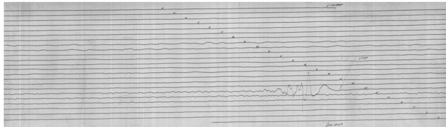
Microbarograph record of the atmospheric nuclear explosion of November 17, 1976 by station Talgar, Kazakhstan,  $\Delta=1065$  km (reads right to left).
