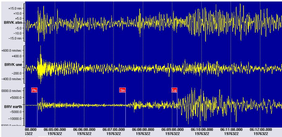
Comparison of station BRVK vertical component seismograms. From top to bottom: atmospheric nuclear explosion of 17 November 1976,  $m_b=4.7$ ; underground nuclear explosion of 29 July 1996,  $m_b=4.9$ ; tectonic earthquake of 30 January 1999,  $t_0=03:51:05.00$   $\varphi^\circ=41.586$ ,  $\lambda=88.455^\circ$ ,  $m_b=5.8$ .
