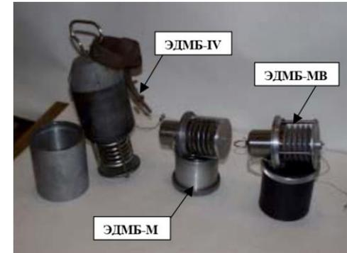
Soviet era microbarograph sensors. The Talgar Observatory, for which we have records, utilized the EDMB-IV sensor at left.
