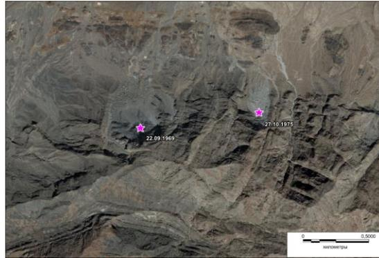
Northern region of Zone B showing slope failures associated with the 22/09/1969 and 27/10/1975 tests (SasPlanet displaying Bing Maps imagery).
