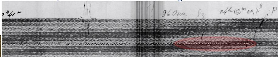
Scan of the vertical component seismogram from the Short period SKM sensor at Charyn, Kazakhstan. This seismogram reads right to left. An clear P wave is marked at 04:02:00.7.
