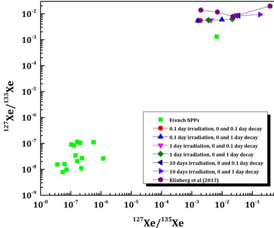
The plot shows French reactors + Klingberg paper + ORIGEN2.1 simulation with thermal neutrons
