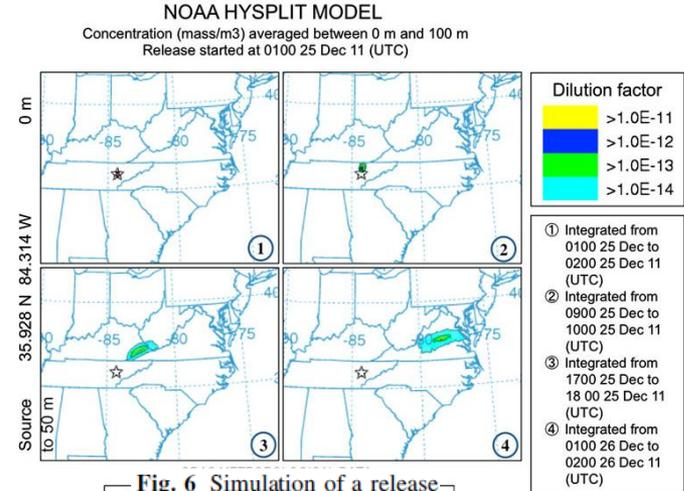
**Fig. 6 Simulation of a release from ORNL HFIR and the plume dispersion to an IMS station**
