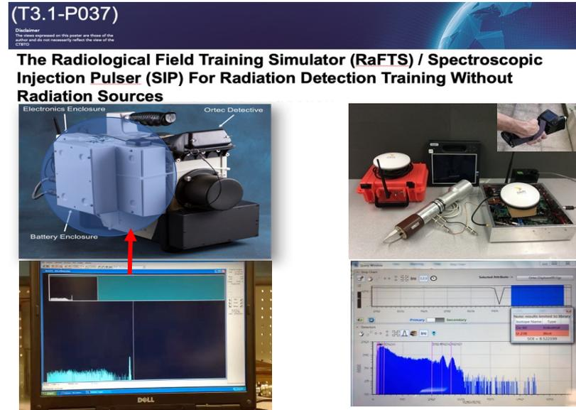
Signals are fed directly into electronics, replicating rad source spectra and encounter physics (e.g.,  $1/r^2$ ...)
