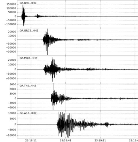
Seismic data of regional station for two days (29/30 July 2019) were provided. Within the data the signature of the NPE 2019 event was manipulated to show somehow explosive characteristics.
