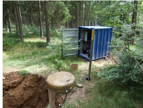
The seismometer remained at the original position in the vault (in the foreground) and was connected to the data acquisition system in the mobile container (in the background).
