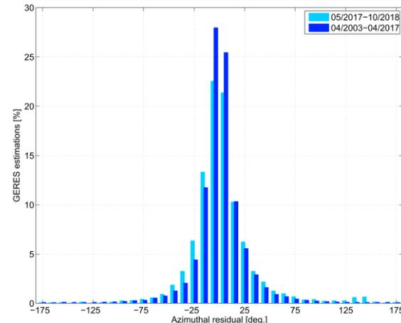
The precision of backazimuth determination was slightly affected by the reduction of array elements from 25 (dark blue) to 10 (light blue). The beam forming with 10 array element shows azimuth variations of less than 29 degree for 80 % of determinations. In comparison, 80% of event determinations with the complete 25 element array have azimuth variations of less than 23 degree.
