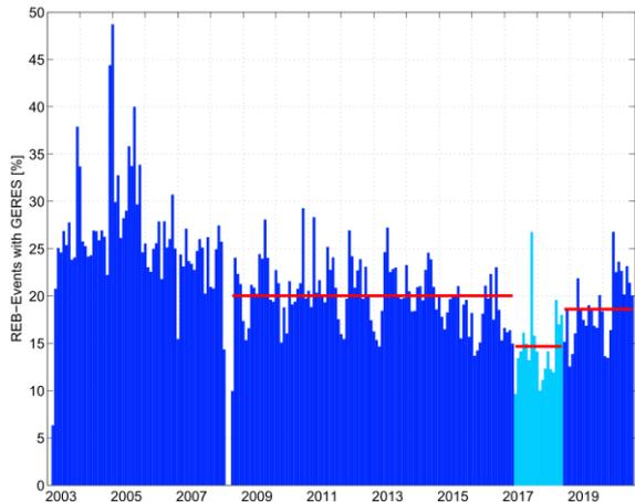
Percentage of REB events with GERES phases on a monthly base between 2003 and 2020. The standard configuration with 25 array elements (dark blue) was temporarily interrupted by the period with a 10 element array in operation (light blue). The mean percentage for the corresponding time intervals are marked in red. It reveals that every fifth event in REB includes GERES phases estimated with 25 array elements, in contrast to only every seventh event with 10 array elements.
