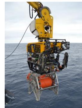
ROV's are equipped with suitable robotic arms, which can enact an underwater repair by disconnecting failed components and replacing them with new ones.
