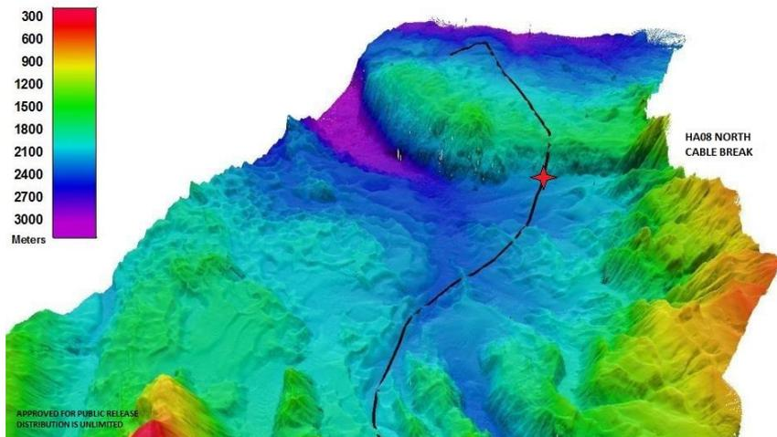
Detail of the undersea topography in the area of the H08N cable break (marked by a red star). The black line shows the route of the hydroacoustic station fibre-optic trunk cable. The colour-scale represents the water depth. Undersea terrain model from US Naval Oceanographic Office.
