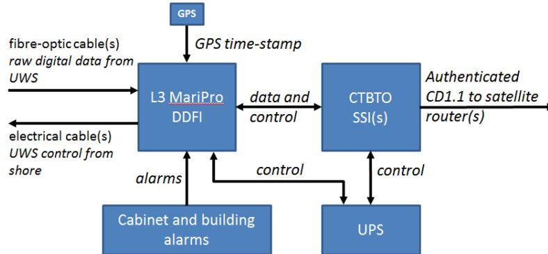
A schematic of the data-flow in the CRF of a cabled HA station.
