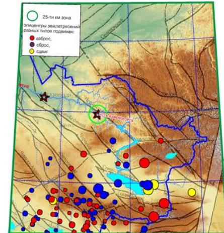
The earthquake epicenters with calculated focal mechanisms on the map of seismic active faults (data provided by Poleshko N.N.)
