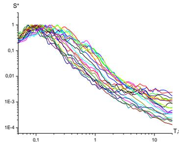
Normalized acceleration reaction spectrum on horizontal components for WWR-K location site.
