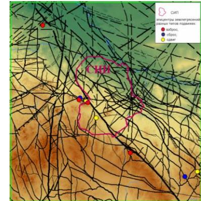
The earthquake epicenters with determined focal mechanisms and type of shift in source (data provided by Poleshko N.N.)
