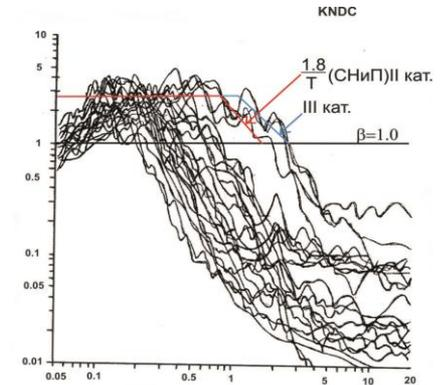
Comparison of dynamicity curve by KNDC with the one by Construction Norms and Rules -2006.
