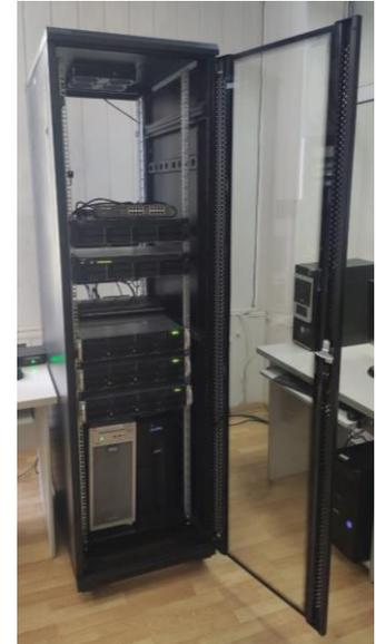
A cluster of three high-performance servers is running a Proxmox Virtual Environment platform. For a fail-safe operation of the system, the cluster uses the distributed file system CEPH, and the data storage system build on RAID technology.
