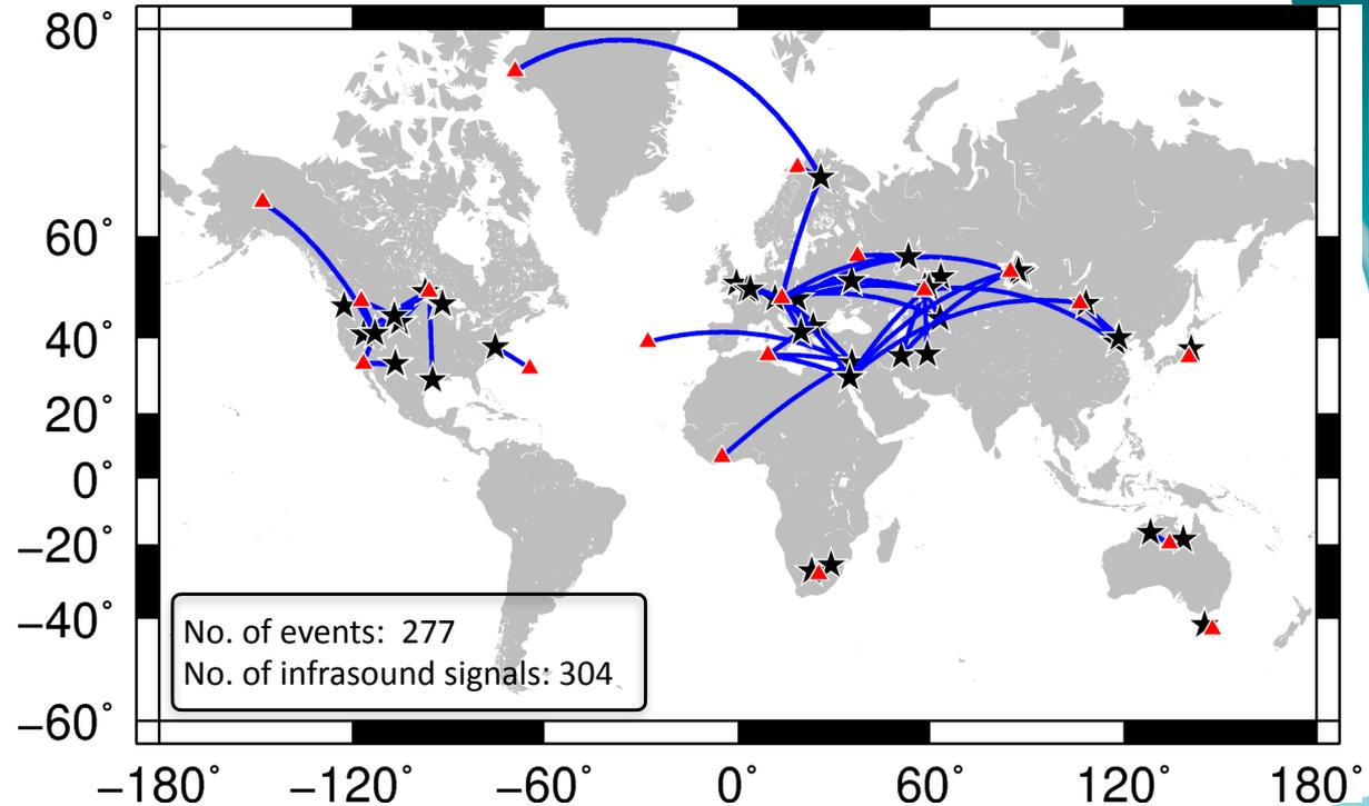
Figure 2. The International Monitoring System (IMS) of the CTBTO stations (triangles) and events (stars) processed. The blue lines indicate the station-event pairs and highlight the dominance of east-west paths.
