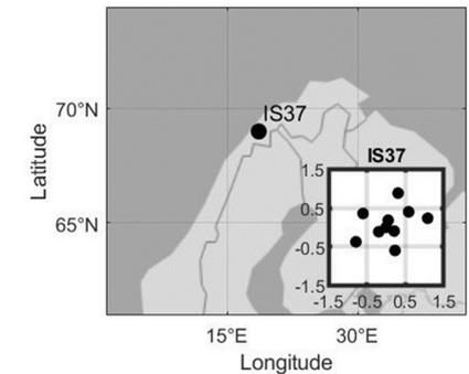
The IS37 array location and geometry.
