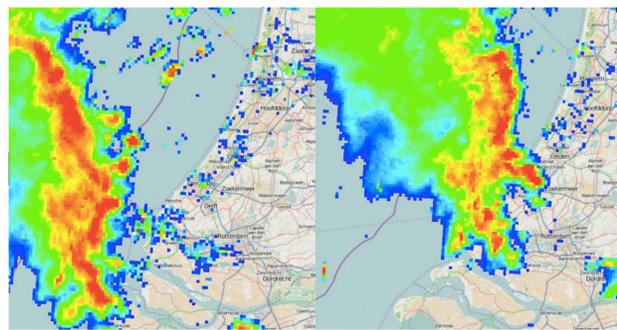
Figure 1: Precipitation image obtained from weather radar at 03:30 and 04:00 UTC, showing the squall-line mesosystem. The storm moves at 75 km/h along the coast.
