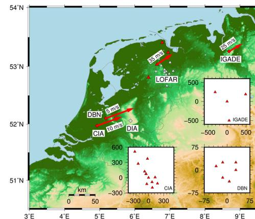
Figure 4: Recordings of the gravity waves on the microbarometer array network in the Netherlands and NW Germany. Array processing allows for the estimation of propagation speed and direction of the gravity waves
