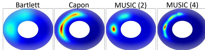
Beamforming results for persistent sources demonstrates the improved resolution of Capon and MUSIC algorithms for identifying multiple, co-incident signals
