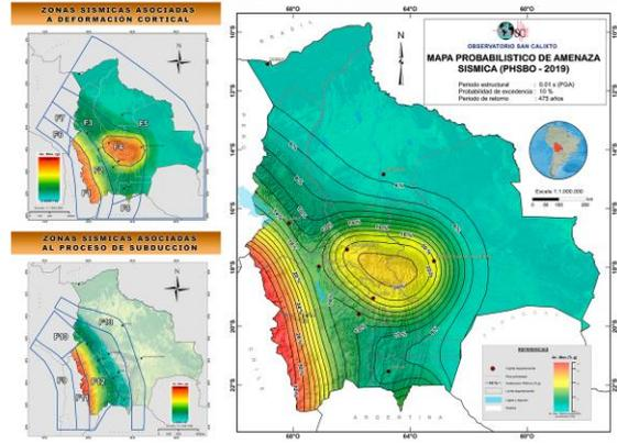
Figure 4 The seismic hazard map for Bolivia at 10% for 475 years. PGAs are expressed on % of g. Small left up side map shows the results for shallow crustal seismicity. Small left down side map shows the results for subduction earthquakes.
