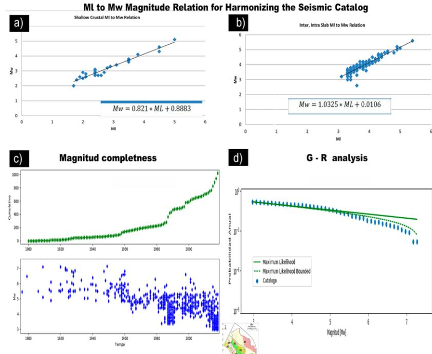
**Figure 4.** a) Shallow Crustal MI to Mw relation regression. b) Subduction MI to Mw relation regression. c) Magnitude Completeness for Shallow Crustal Seismicity. d) G - R plot for Shallow Crustal Seismicity.
