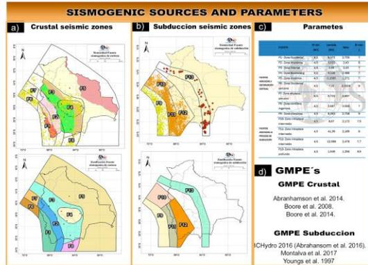
Figure 3 a) Shallow Seismicity M-5 distributed under the geomorphologic map and zonation. b) Interface, subduction and deep Seismicity M-5 and Zones delimitation for the analysis. c) Parameters taken into account with their magnitudes, lambda and beta values. d) GMPE's used in this work.
