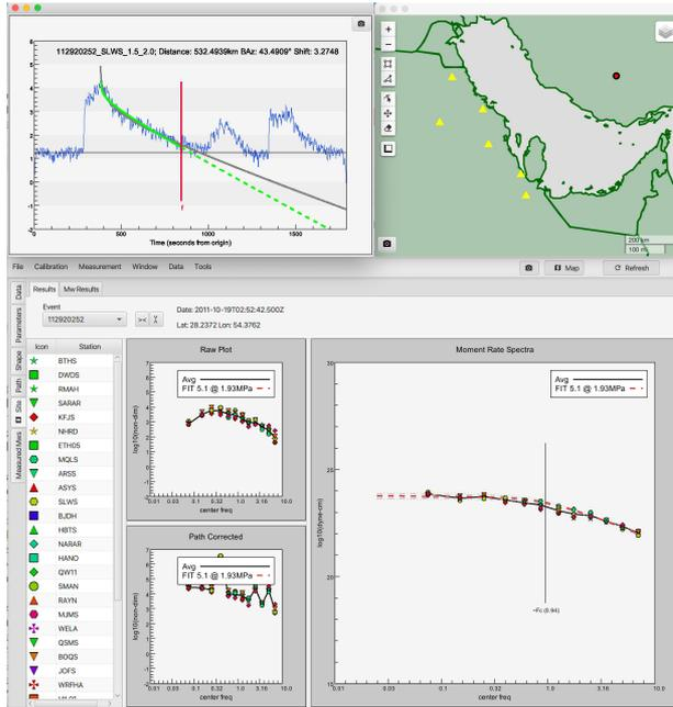
**Figure 6** An example source spectra of coda calibration result from the Zagros subregion
