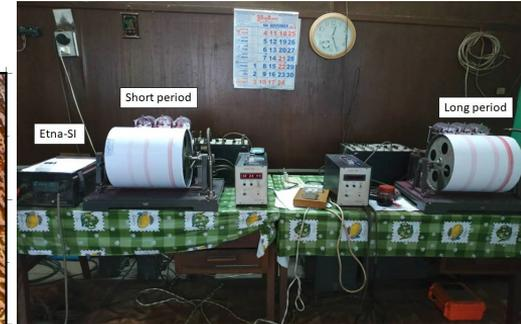
**Katsujima analog seismographs in Yangon seismic station**
