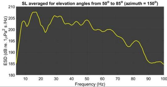
*Energy spectral density levels of the received signals at H10N (average of high SNR signals from identified shots).*
