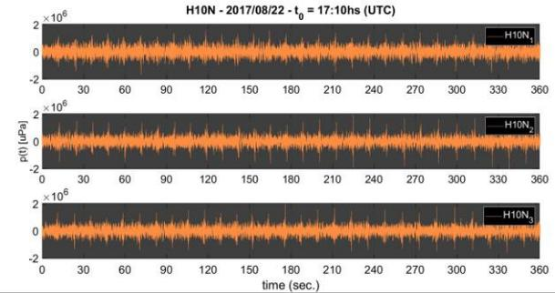
**Materials:** A selection of signals with high signal to noise ratio (SNR) recorded at HA-IMS station and back-azimuths compatible with ground-truth airgun seismic survey.
