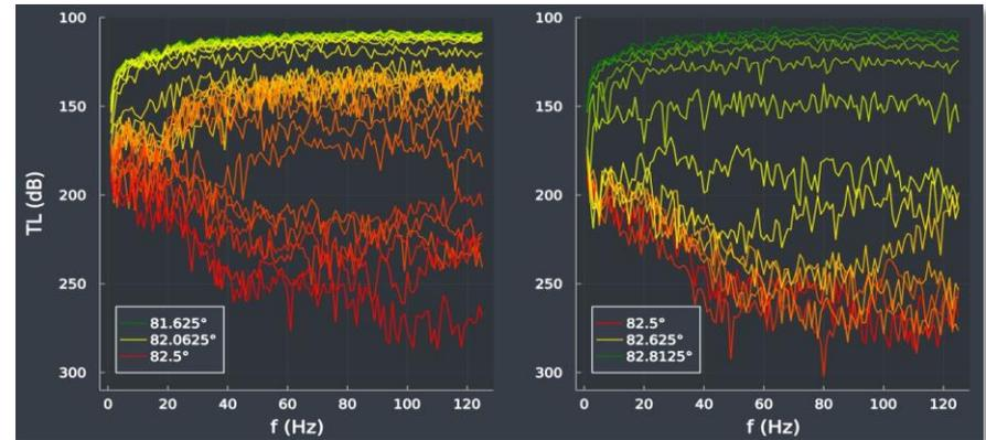
*Strong variations vs. azimuth from H10N is observed principally due to bathymetric features in the acoustic path.*
