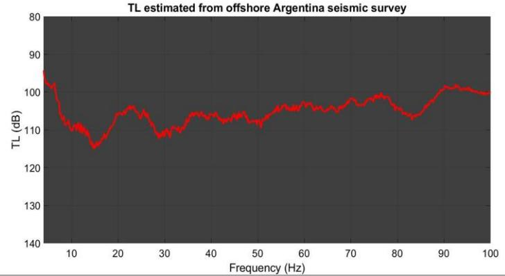
The *TL* estimation errors are about 5 dB due to uncertainties associated to variability of signal's amplitude and modelled  $ESD_{source}$ . Further work is required in order to compare results with *TL* models and correlate  $L_{rec}$  variations with propagation effects or actual variations of the source energy and its coupling in the sound channel.
