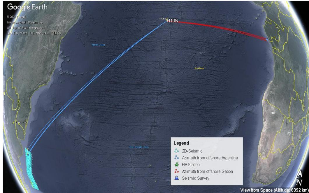
*Examples of two airgun seismic surveys recorded at H10N station. The geodesic paths obtained for the back-azimuths computed from high SNR signals are shown from H10N to seismic surveys areas for two cases: **1)** offshore Gabon ~2760 km and 81.8 deg. (red lines) ; **2)** offshore Argentina ~5250 km and 223 deg. (blue lines).*
