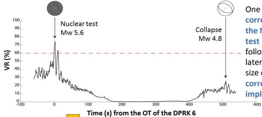
One main VR peak corresponding to the Mw5.6 nuclear test (explosion) followed 8min30 later by a smaller size event (Mw4.8) corresponding to an implosive source
