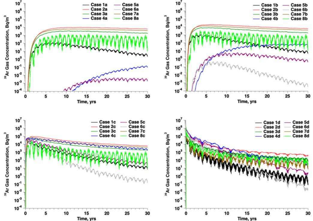
Predicted <sup>39</sup>Ar concentrations in the model domain at various times. This illustrates the influence that a much more highly-permeable host rock (1a) can have compared to a lower-permeable host rock (6a).
