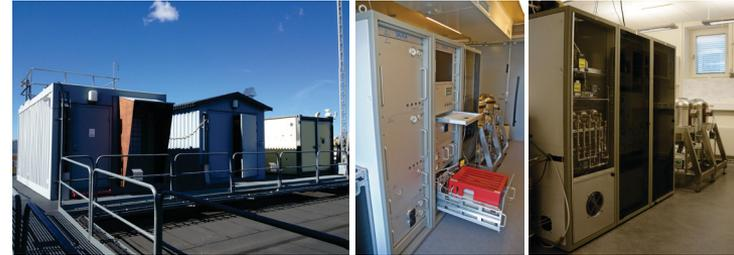
Two systems are co-located at the IMS RN63 (left) site in Stockholm, Sweden: SEX63 a SAUNA II system (the IMS station, center picture) and SAX63, the first SAUNA III (right). SEX63 was installed at the site in 2005 and the SAUNA III system started measuring in 2017.
