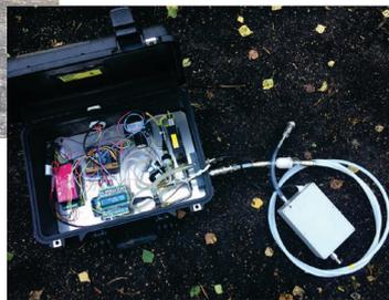
The soil gas was sampled into balloons (typically at 6 l/min). The sample sizes ranged from 1 to 5 m<sup>3</sup>, but most samples were 2-3 m<sup>3</sup>. Sampling was carried out during day time only. No extra traps for removal of CO<sub>2</sub> nor water was used. After the collection was completed the gas was compressed into scuba bottles and transported to the laboratory in Stockholm for analysis.
