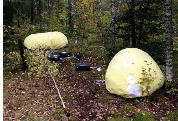
Balloons being filled with soil gas extracted using FOI samplers (seen in the middle of the photo). The sampling rate is approximately 6 L/min at a sampling depth of approximately 3 m.
