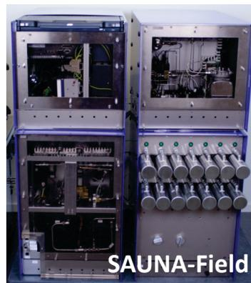
The soil gas from the scuba bottles was processed in SAUNA-Field and measured either directly or transferred to the SAUNA-Lab system via archive bottles.
