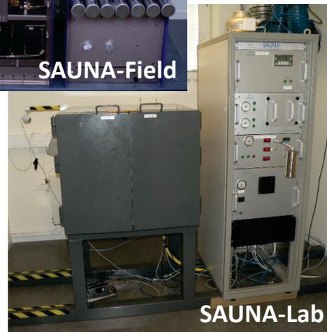
Argon samples were "collected" into bags both directly on site and from the drain of SAUNA-Field system. The samples were then shipped to the University of Bern for analysis.
